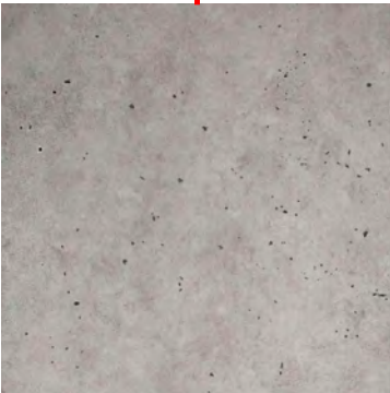
OFF FORM CONCRETE Class 2 finish structural elements, facade planters
